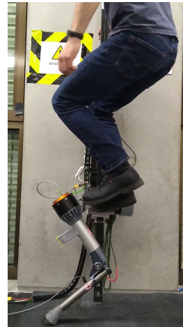
Fig. 7: Leg prototype sustaining a 65 kg person.
