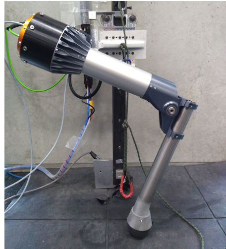
Fig. 1: Robotic leg prototype mounted on a linear guide.
