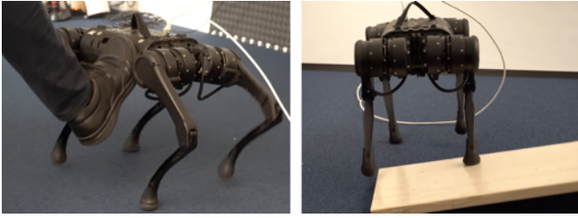
Fig. 3. We pushed (left) and disturbed the Unitree A1 robot by putting a plate under its feet (right) while it was performing a trot gait.
