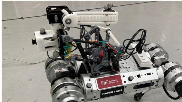
Fig. 1. The prototype of proposed neck design with a Mini Cheetah [10].
