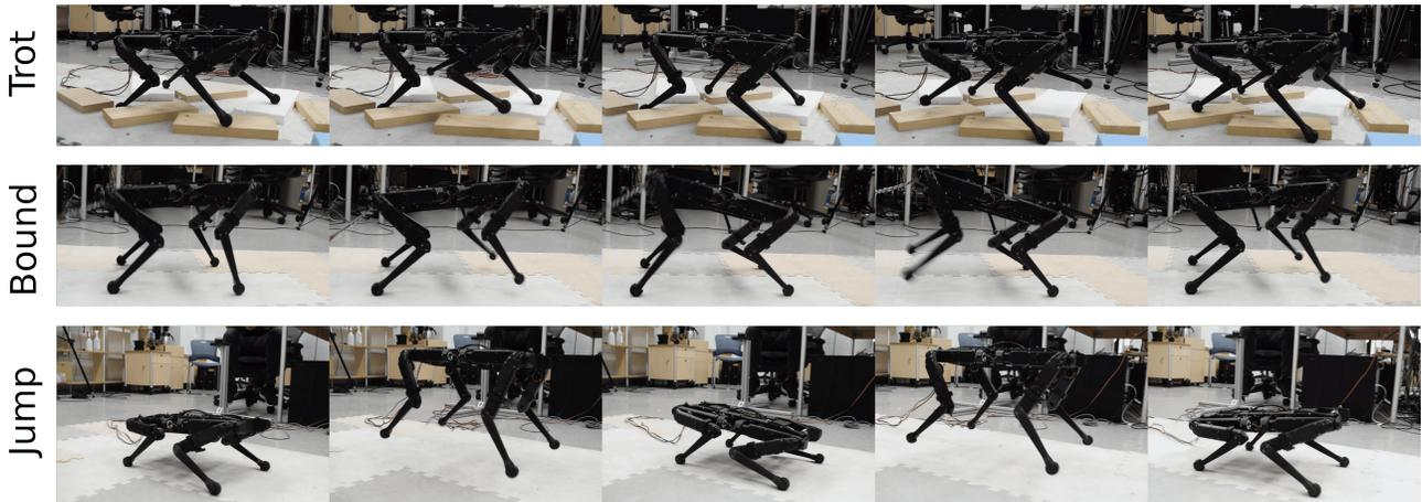
Fig. 2: Different motions demonstrated on real robot with solo12.
