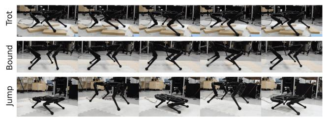
Fig. 2: Different motions demonstrated on real robot with solo12.
