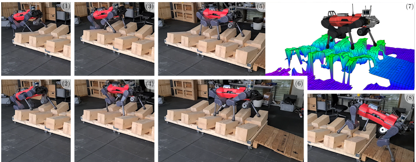
Fig. 7. ANYmal traversing a stepping stone parkour made of inclined wooden bricks using a trotting gait. The commanded heading velocity is 0.4 m/s. The dimensions of each brick are 20\text{ cm} \times 20\text{ cm} \times 50\text{ cm} and the gap between any two adjacent bricks measures 20 cm. Due to the inclined surfaces, the model assumptions are not perfectly satisfied in this experiment. Picture 7 shows the visualization of the robot along the raw elevation map.
