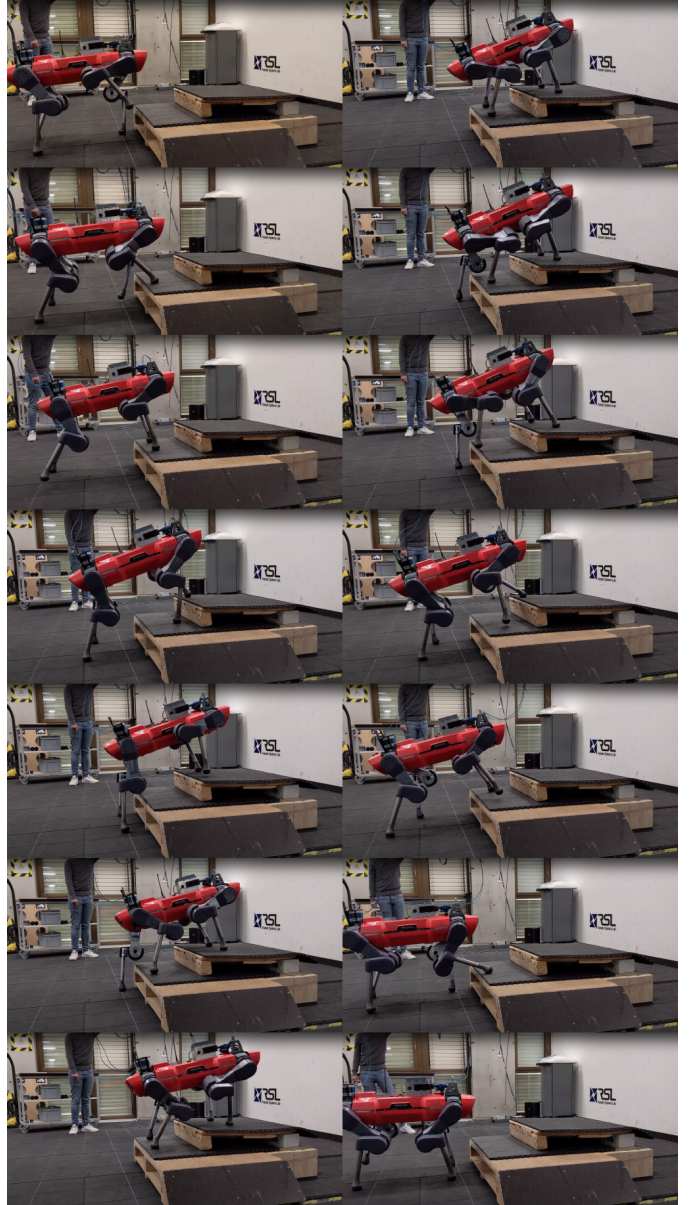
Fig. 3. Experimental verification of the GP+NMPC+WBC combination performed on the quadrupedal robot ANYmal in a laboratory setting. All frames are extracted from a single continuous trial, however, the left column corresponds to first stepping up onto the obstacle, while the right column to the respective descent.
