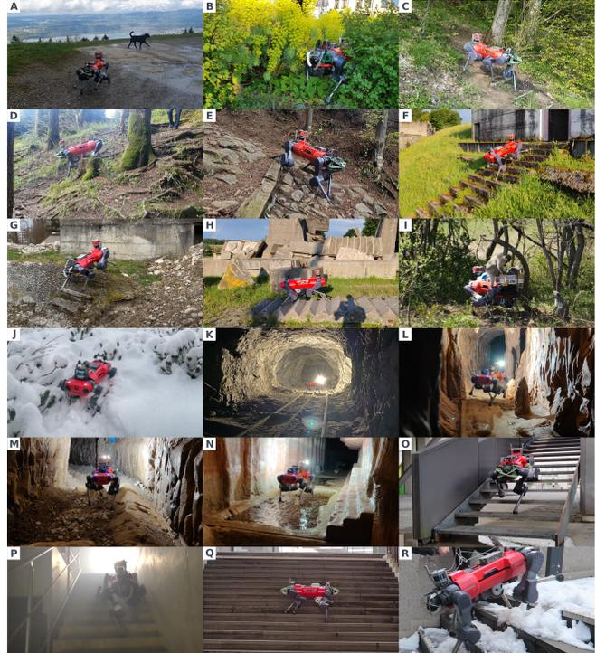
Fig. 1. Robust locomotion in the wild. The presented locomotion controller was extensively tested in a variety of complex environments over multiple seasons. The controller overcame a whole spectrum of real-world challenges, often encountering them in combination. These include slippery surfaces, steep inclinations, stairs, snow, and vegetation with degraded exteroception. The controller traversed these environments with zero failures.
