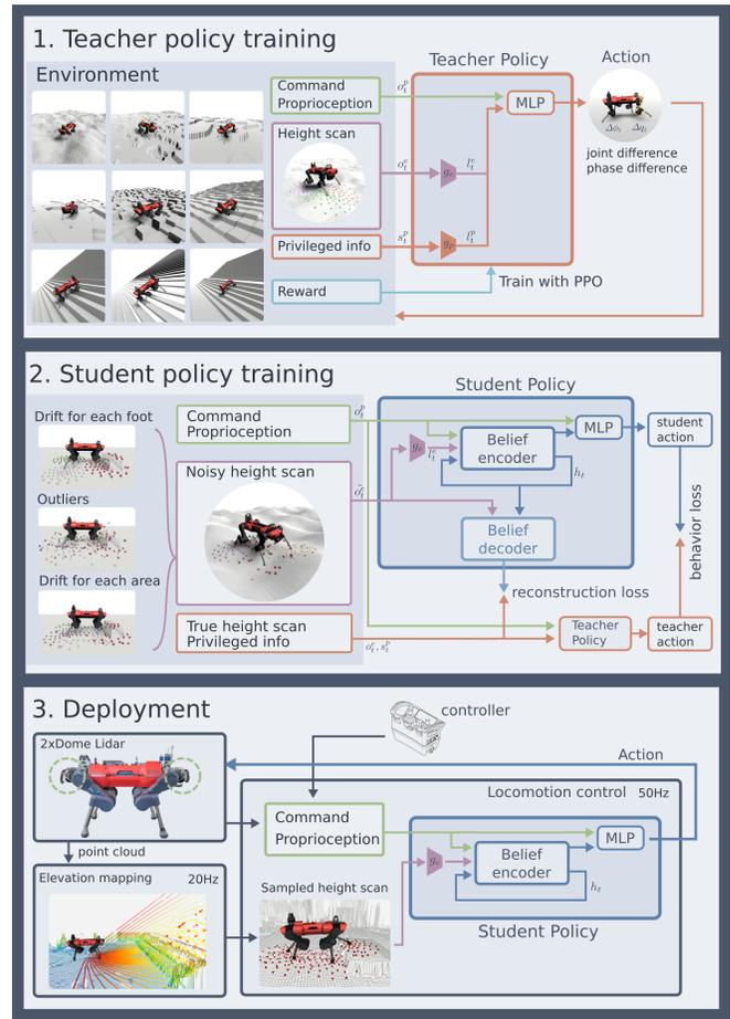
Fig. 2. Overview of the training methods and deployment. We first train a teacher policy with access to privileged simulation data using reinforcement learning (RL). This teacher policy is then distilled into a student policy, which is trained to imitate the teacher’s actions and to reconstruct the ground-truth environment state from noisy observations. We deploy the student policy zero-shot on real hardware using height samples from a robot-centric elevation map.
