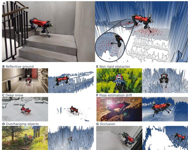
Fig. 3. Our locomotion controller perceives the environment through height samples (red dots) from an elevation map (A). The controller is robust to many perception challenges commonly encountered in the field: missing map information due to sensing failure (B, C, G) and misleading map information due to non-rigid terrain (D, E) and pose estimation drift (F).
