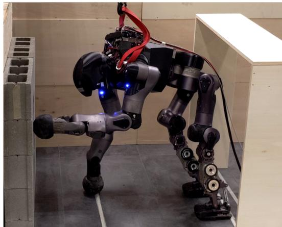
Fig. 1: The COMAN+ humanoid robot standing up taking advantage of a vertical wall placed in front of it.
